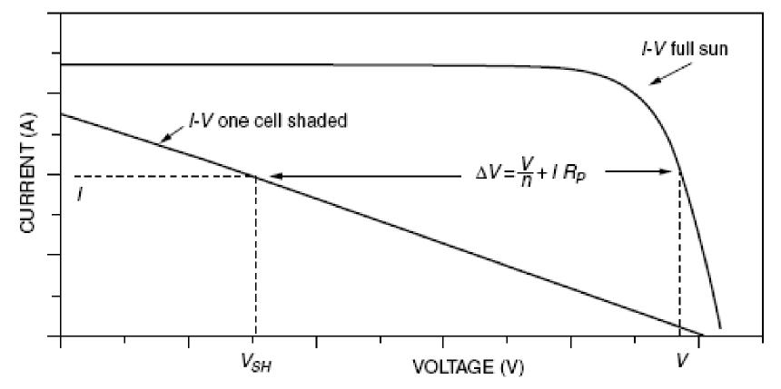
Effect of shading one cell in an *n*-cell module. At any given current, module voltage drops from V to  $V - \Delta V$ .
