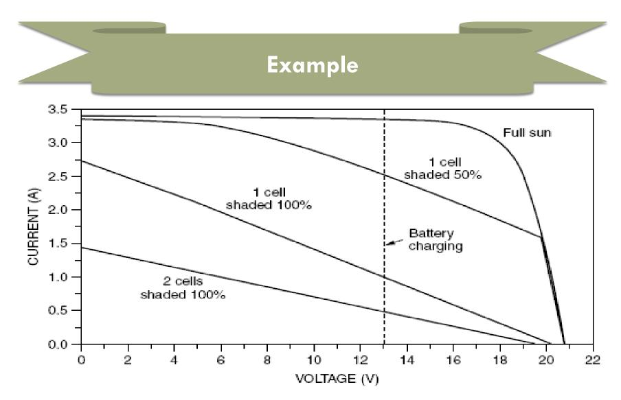
Effects of shading on the I-V curves for a PV module. The dashed line shows a typical voltage that the module would operate at when charging a 12-V battery; the impact on charging current is obviously severe.
