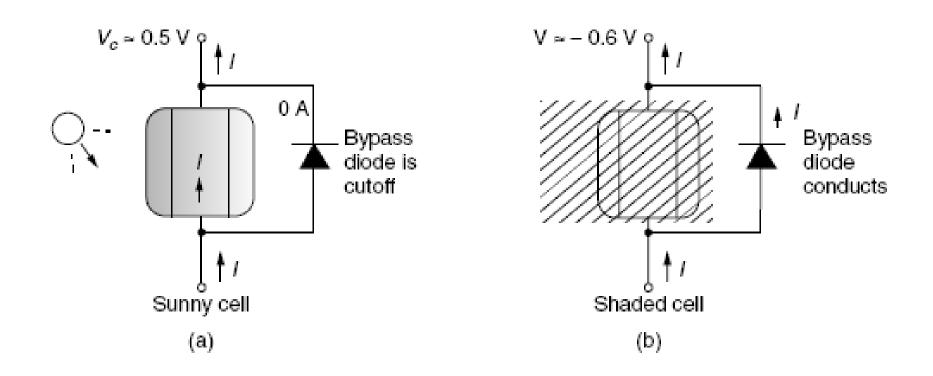
Mitigating the shade problem with a bypass diode. In the sun (a), the bypass diode is cut off and all the normal current goes through the solar cell. In shade (b), the bypass diode conducts current around the shaded cell, allowing just the diode drop of about 0.6 V to occur.
