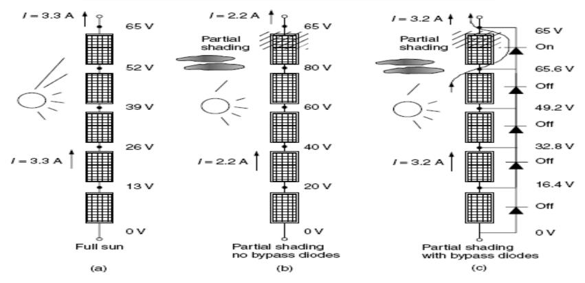
Showing the ability of bypass diodes to mitigate shading when modules are charging a 65 V battery. Without bypass diodes, a partially shaded module constricts the current delivered to the load (b). With bypass diodes, current is diverted around the shaded module.
